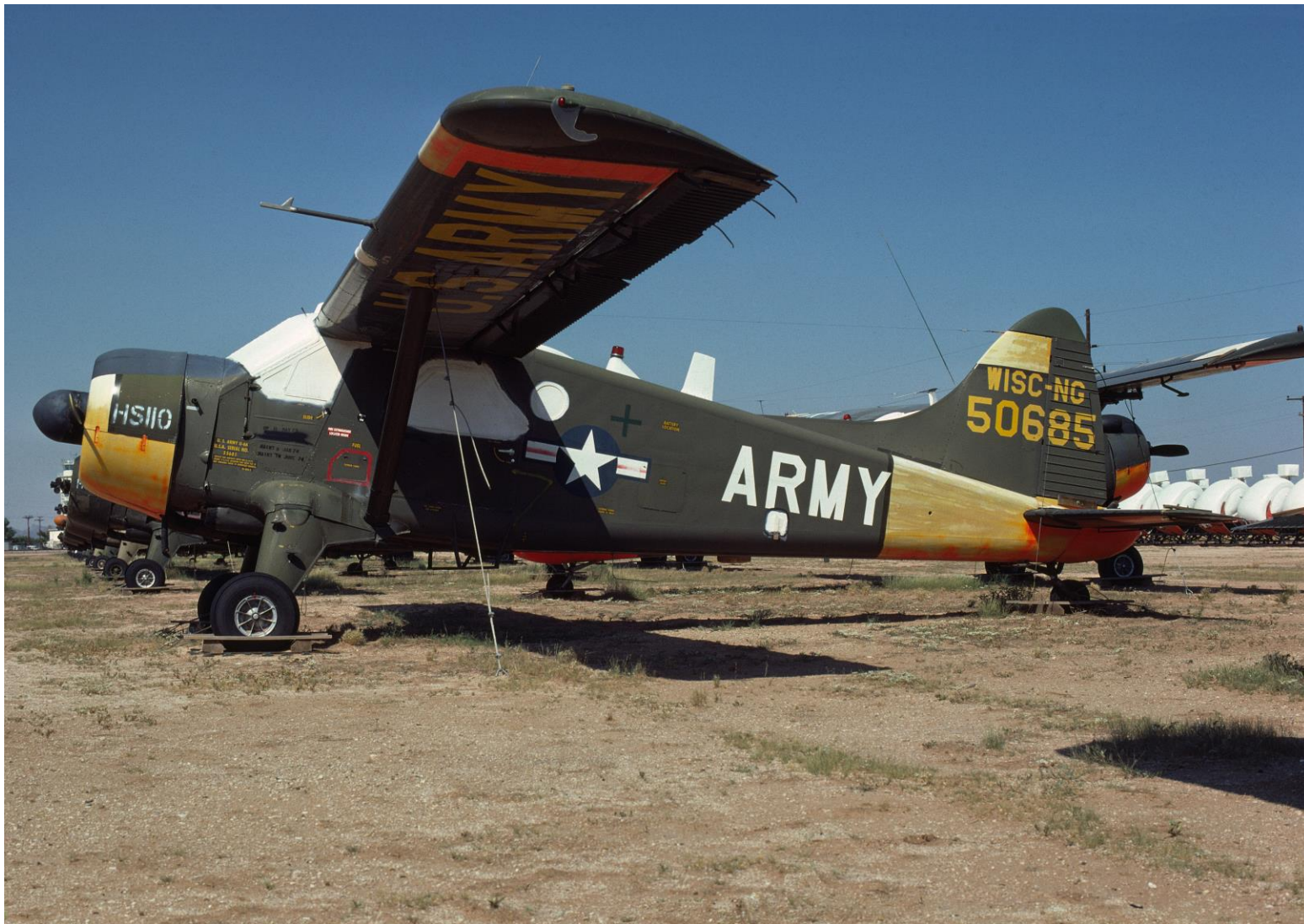
55-0685 (903) ex Wisconsin National Guard, with white spray-lat coating to keep out the heat and dust while parked at MASDC for four years exactly.
